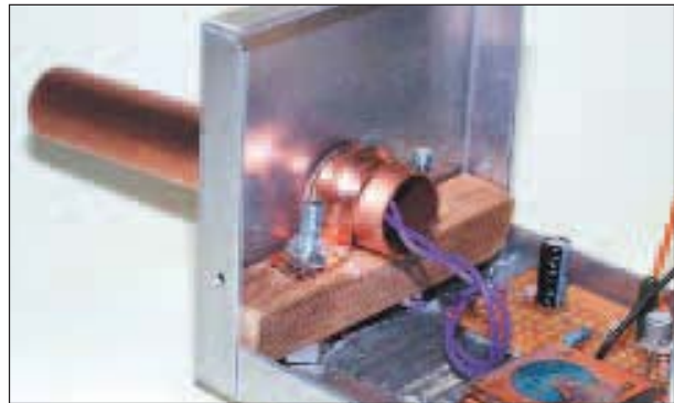
Fig.5. Insulating and wiring the microphone insert (a), end view showing insert "plugged" into the copper pipe (b) and the Mic. insert recessed in the copper tubing (c)
